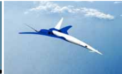
This “Icon-II” future aircraft design concept for supersonic flight over land comes from the Boeing Company.
